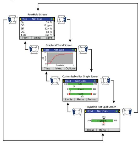
Use function keys F1 and F3 to configure and define options (if available) such as alarm points, parameters to be monitored, timing parameters, etc. Components of the graphics screens are identified in the sections that follow.
