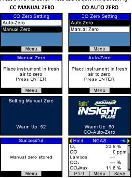
By default, the Fyrite<sup>®</sup> INSIGHT<sup>®</sup> Plus automatically zeroes all sensors on ambient air when the instrument is turned on.
