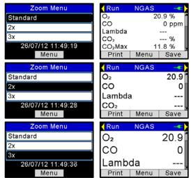
The operator can scroll through the complete list of data (using the UP ( $\triangleq$ ) and DOWN ( $\blacktriangledown$ ) arrow buttons) regardless of the zoom level.
