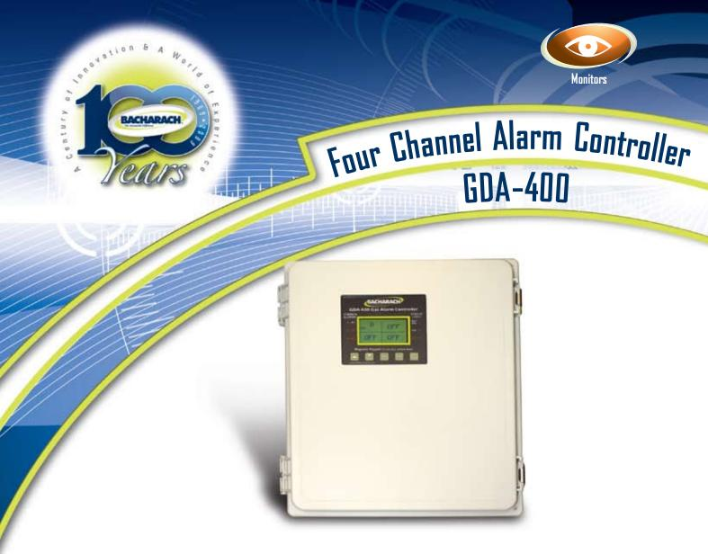
Bacharach's GDA-400 four channel controller is designed to provide simultaneous display and alarm functions for up to four monitors with 4-20 mA inputs. A graphic LCD displays monitored data as gas type and concentration, bar graphs and 30 minute trends. Three adjustable alarm levels are provided per channel. Relay outputs allow control of audible and visual alarms, strobes, horns, and other alarm events.
