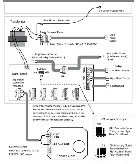
Figure 11. Wiring (6-Channel, Dual-Alarm Unit Shown)
