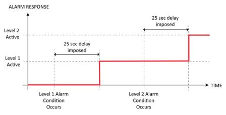
Figure 17. Alarm Response (Dual-Level Alarms)
