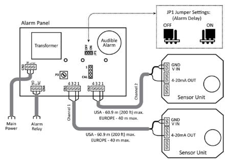
Figure 8. Wiring (2-Channel, Single-Alarm Unit Shown)
