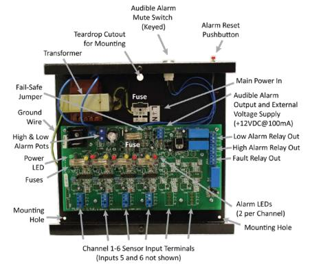
Figure 4. 6-Channel, Dual-Alarm MGS Controller
