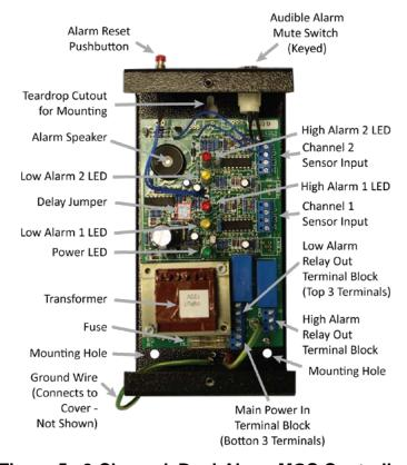
Figure 5. 2-Channel, Dual-Alarm MGS Controller
