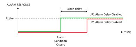
Figure 16. Alarm Response (Single-Level Alarms)
