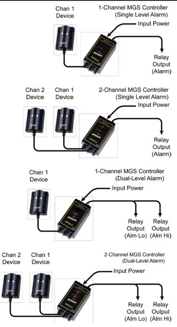
Figure 1. Sample Configurations (1,2-Channel)
