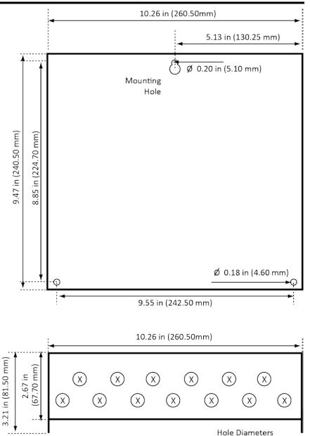
Figure 7. Mounting Dimensions (6-Channel Unit)
