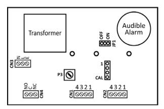
Figure 12. Hardware PCB Layout (2 Channel, 1 Alarm)
