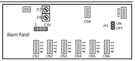
Figure 15. Hardware PCB Layout (6 Channel, 2 Alarm)
