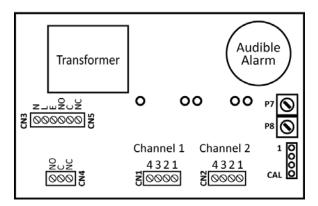
Figure 13. Hardware PCB Layout (2 Channel, 2 Alarm)
