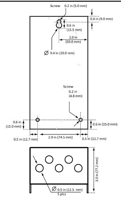
Figure 6. Mounting Dimensions (2-Channel Unit)
