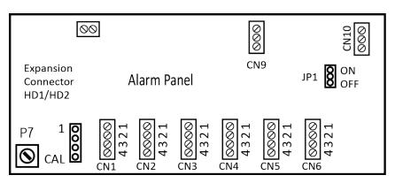
Figure 14. Hardware PCB Layout (6 Channel, 1 Alarm)
