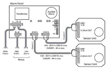
Figure 9. Wiring (2-Channel, Dual-Alarm Unit Shown)
