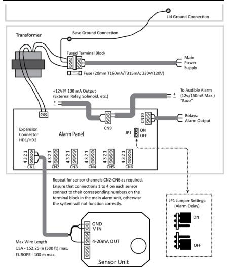
Figure 10. Wiring (6-Channel, Single-Alarm Unit Shown)
