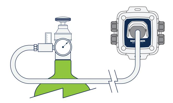
2. If using a variable flow regulator, adjust the gas flow to approximately 0.3 L/min.
