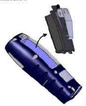
To replace alkaline batteries, remove the cover plate on the battery pack by rotating the two screws a quarter-turn counterclockwise. Pull out the old batteries and replace them with new batteries in the same orientation (see illustration).
