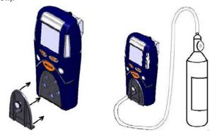
When the sensor has been adjusted, the monitor will display a prompt for the next gas to be applied.
