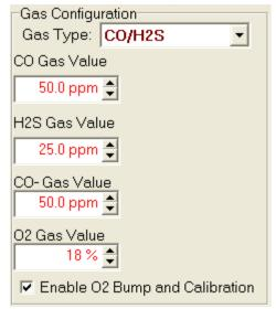
The IQ System will automatically fail any detector that is processed when the calibration gas type fails to match the sensor type.
