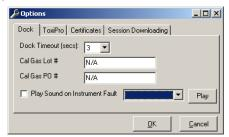
The Dock Timeout Setting controls the amount of time that needs to pass after connection between the dock and the PC is lost before the system will notify you that the connection has been lost. Options are given in whole numbers between 1 and 10 seconds. To change the setting, click on the arrow to the right of the timeout setting to access the list and select the new setting.
