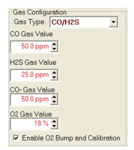
To change the gas type, click on the down arrow to the right of the gas setting and select the new gas type.
