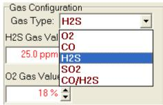
Once the gas type is chosen, enter the calibration gas composition, including the values for any toxic gases in the cylinder in terms of parts-per-million (ppm) and the oxygen level in terms of percent volume (%). To change a gas value use the arrows to the right of the gas value input box to increase or decrease the value until it matches the value given on the gas cylinder.
