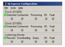
For docks in Listening Mode, if a single fault is detected on any of the docks, the dock LED will turn grey and the Fault LED will turn red.
