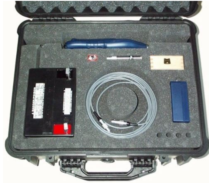
CEL-6723 Environmental kit case for CEL-480 Logging sound level meter
