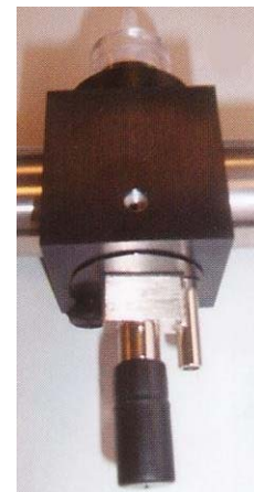
Respirable adapter fitted to Microdust pro probe
