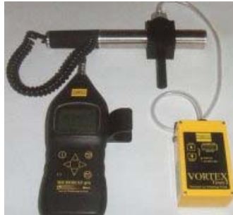
Microdust pro RDM with gravimetric dust adapter and pump
