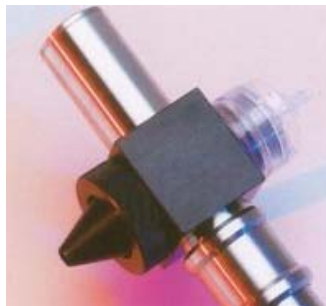
Size selective dust adapter with PUF filters
