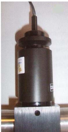
Aspirated adapter fitted onto Microdust pro probe
