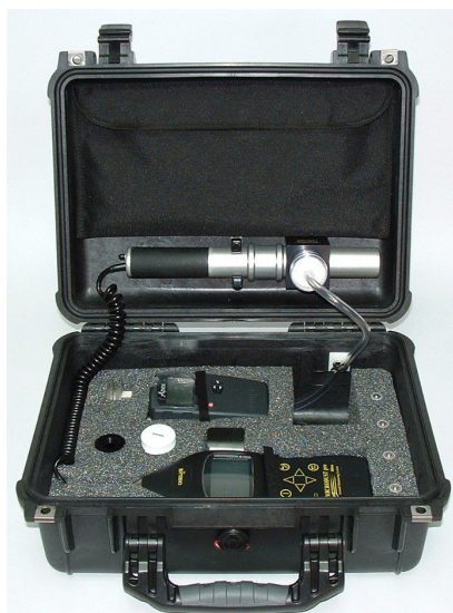
The 176170D Dust Detective weatherproof kit with Microdust Pro dust monitor and Apex Lite pump
