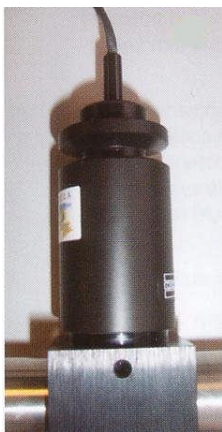
Aspirated adapter fitted onto Microdust Pro probe
