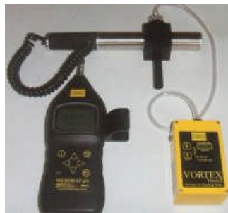
Microdust Pro RDM with gravimetric dust adapter and pump (any pump can be used)
