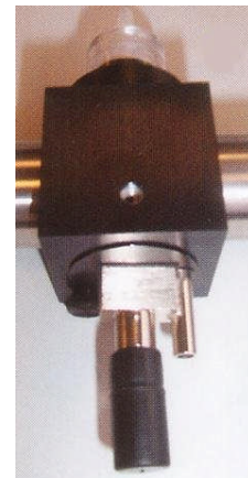
Respirable adapter fitted to Microdust Pro probe
