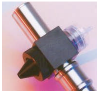
Size selective dust adapter with PUF filters
