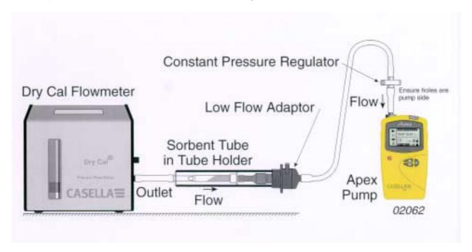
Please note the attachment may also be made to a dry flow meter or burette in the same manner. (Here a stopwatch will be required to measure the time to sample a specific volume.)
