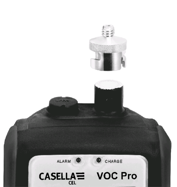
Figure 14. Replacing the Inlet Filter
