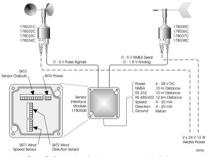
Figure 5: Connections for the anemometer and windvane
