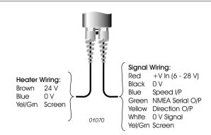
Figure 4: Connections for Wind-vane versions with heaters
