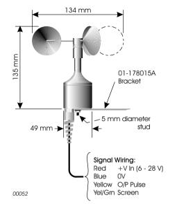
Figure 1: Anemometer wind speed sensor
