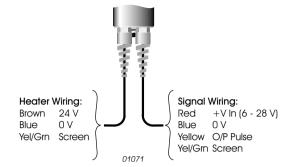
Figure 2: Connections for anemometer versions with heaters
