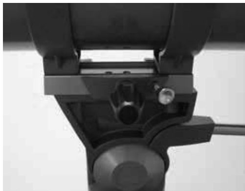
Fig. 2-12 Mounting Knob & Safety Screw in the dovetail bracket
