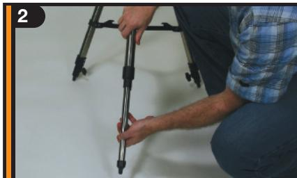
To set up the tripod, spread the legs outward until they are fully extended. Extend each of the three tripod legs down 6-12".
