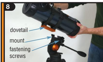
Next slide telescope tube into the mount. Be sure to back out fastening screws to allow enough clearance for the dovetail
