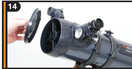
Remove the lens cap from the front of the telescope before you begin observing.
