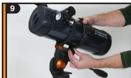
Center dovetail in the mount and tighten fastening screw. For added security tighten the angled lock down screw next to the fastening screw.
