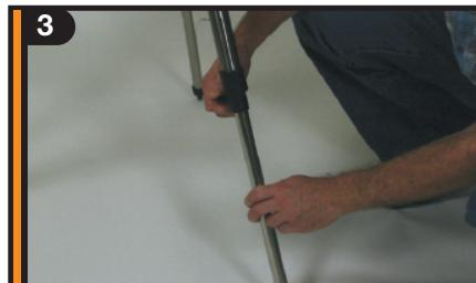
Use the three tightening screws located at the bottom of each leg to secure the extended legs in place.
