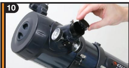
Loosen the set screw on the focuser. Remove the plastic cap covering the end of the focuser.
