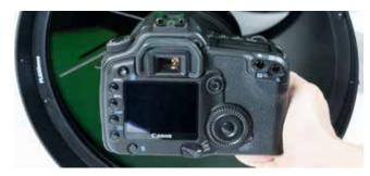
4. Finish threading the retaining ring onto the telescope. Turn until the camera adapter is snug against the telescope. Do not over tighten! Camera orientation can be adjusted later.
