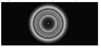
6. Adjust the telescope collimation if needed by slightly loosening a 3mm socket head screw, and tightening the paired 2mm socket head screw. The screws work as push/pull, tightening one requires loosening the other. Always adjust one pair of screws at a time.
