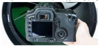
4. Finish threading the retaining ring onto the lens group housing. Rotate the ring until the camera adapter is snug against the housing. Do not over tighten! Camera orientation can be adjusted later.
