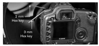
7. If the star pattern is thin on one side, adjust the collimation screws so that the star moves towards the thin side, then adjust the position of the astrograph to re-center the star. Repeat this until the defocused star image is concentric.
