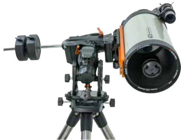
Figure 9.2 One side of DEC mechanical limit
