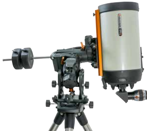
Figure 6 Balancing the mount
