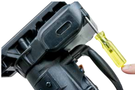
Figure 12 Removing the gear cover
