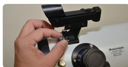
4. Now slide the dovetail bar on the bottom of the optical tube into the clamp assembly on the top of the mount. Be sure to back out the fastening screw to allow enough clearance for the dovetail bar.
