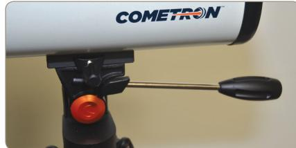
12. Turn the panning handle of the mount counterclockwise to loosen the altitude (up & down) clutch. Use the pan handle to move the telescope until your target appears in the finderscope. When you have your target in the field of view of the telescope eyepiece, tighten the altitude lock nut.
