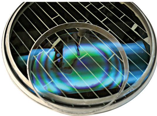
FIGURE 7. Matchplates use interference fringes to check the radius and smoothness of the correction. In this picture, a corrector blank is attached to a master block. The matchplate rests on top; interference fringes appear as green and blue circles. The circular pattern indicates a difference in radius.
