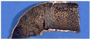
Wall thinning is the natural result of pressure or movement of materials through curved portions of pipelines
