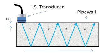
When using MultiECHO™; four readings are required before the UT5000 displays a value. With MultiECHO™ an inspector can be confident that the reading stored is accurate and unaffected by couplant or surface interference.
