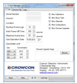
**Gas Bottle Fields:** Users can program in detailed information about their calibration gas. Expiration Date and Bottle Lot # will appear on each test record. If the expiration date is set to today's date, that field will remain blank on the test record.
