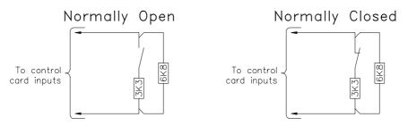
Monitoring of outputs needs to be done by using an additional relay, either on a DI-944 relay card or using rail mounted relays external to the rack if the switching current is more than 1 amp. The method of monitoring output devices relies on a polarity reversal scheme.
