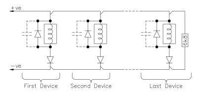
Once again, the capacitors are optional and the power diode must be capable of handling the maximum operational current of the device. In this arrangement only the loop cabling can be monitored, not the devices themselves.
