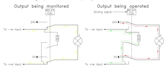
As can be seen from the diagram above, when the device is being monitored the monitoring signal goes through the field cabling and through the device. When the device is in use then the polarity reverses and the monitor card is put into alarm by switching in the 3.3 k $\Omega$  resistor.
