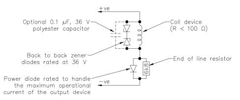
In the above diagram the optional 0.1  $\mu$ F, 36 V capacitor need only be fitted as extra protection against RFI or EMF spikes which may harm the control card when high inductance items are being monitored. The pair of Zener diodes act as back-EMF diodes which will not conduct until the back-EMF voltage exceeds 36 V dc, thus forcing the 24 V monitoring signal through the coil. If
