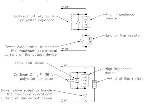
If more than one of the devices to be monitored are on a loop then the following loop scheme must be employed.
