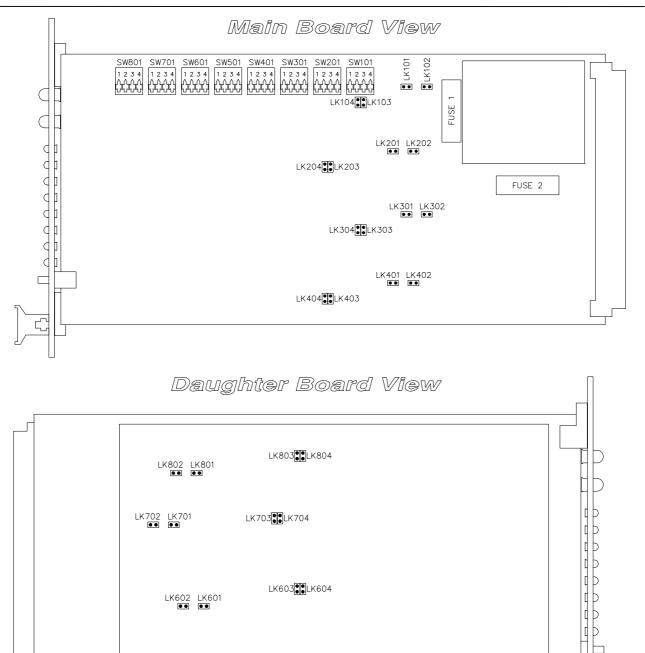
Links LK*n*03 and LK*n*04 are a pair and should be fitted vertically for normally open input circuits and horizontally for normally closed inputs, as shown.
