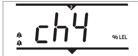
Figure 3.3 Example system in alarm
