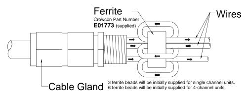
At minimum, the following cables require this application: Mains Power, Channel Input, and Audible Visual Alarm
