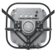
When unpacking the composite framed Detective+ IR for the first time, the three legs will be in the folded position.
