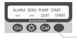
Press the UNMARKED button to enter the START submenu
