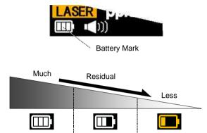
When the battery power of the battery pack is lost until this product doesn't operate, the empty screen shown on the right will be displayed, and there will be an alarm.
