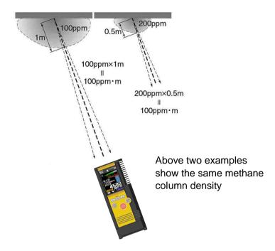
In addition, this product does not respond in principle to gases other than methane (butane, propane, etc.). This product cannot perform detection in places where detection laser beam cannot reach, such as the opposite side of a wall or underground.
