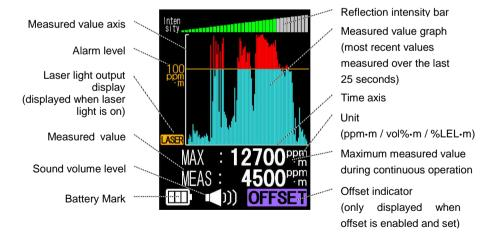
When the remaining battery level is shown in the figure on the right, the power will switch off in approx.15 min. If this symbol appears, recharge the battery pack. (See "4.1 Charging Battery Pack")
