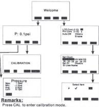
Under the "REC" function. Curr. means the current value. There are total 11 units could be selected under SET function. The selectable units are psi/Inch of H2O/bar/mbar/mm of Hg/ Inch of Hg/oz/inch2/Kg/cm2/kPa/Ft of H2O/cm of H2O
