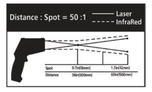
large as the spot size. As the distance (D) from the object increases, the spot size (S) of the area measured by the meter becomes large. The relationship between distance and spot size is shown above. The focal point is 36" (914 mm). The spot sizes indicate 90% encircled energy.
