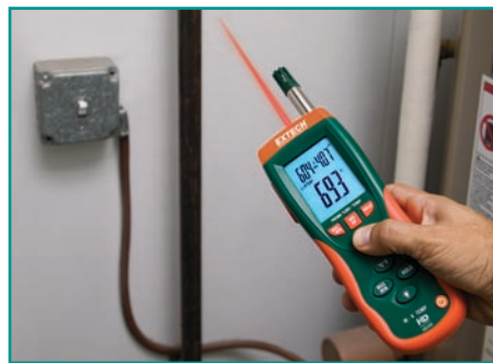
Patented non-contact InfraRed Thermometer technology built into a Hygro-Thermometer like the HD500 is perfect for Home inspection applications.
