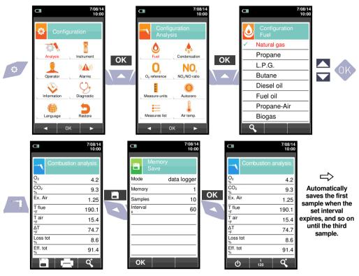
In case the automatic print mode is set then the average analysis printing start automatically. Conversely, after the sampling of the third analysis, the average analysis is shown, so that it can be sent to the printer as explained in the following.
