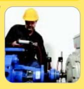
user you are given step-by-step instructions on the display through the entire measurement procedure. Even though the technology inside is rather advanced, the measurement principle is straightforward. It is based on the "reverse indicator method" with two laser/measuring units mounted on each side of the coupling.
