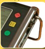
Countersunk connectors, well protected against external damage.
