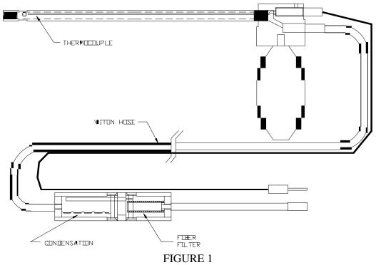
The probe assembly consists of the following components:
