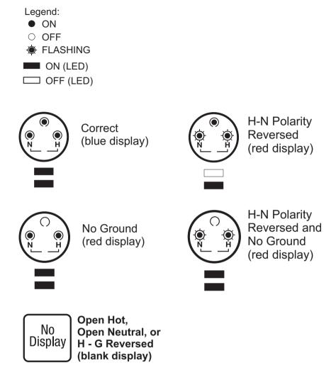
**Note:** For open HOT, open NEUTRAL, and H-G polarity reversal conditions, the meter is completely switched OFF and therefore no display or LED status is available.
