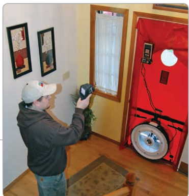
Thermal imaging used in conjunction with blower door pressurization accentuates air leak patterns and other energy efficiency issues.
