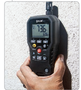
FLIR MR77 features a pinless moisture sensor and a wired pin probe
