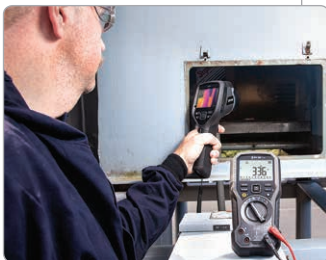
Automatically annotate thermal images with critical load data
