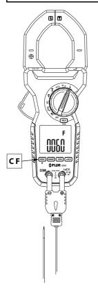
Figure 5.8 Thermocouple Temperature Measurements.
