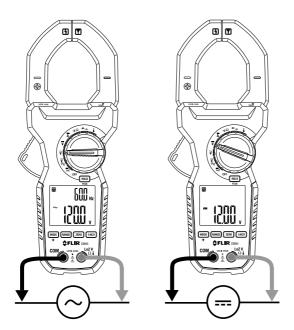
Figure 5.2 AC Voltage (left) and DC Voltage (right) Measurement Setups
