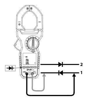
Figure 5.6 Diode Testing. Note the two test positions, forward and reverse bias.
