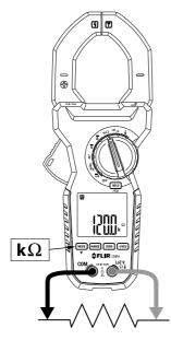
Figure 5.4 Resistance Measurement Setup.
