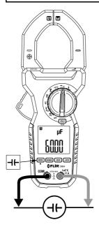
Figure 5.7 Capacitance Measurement Setup.
