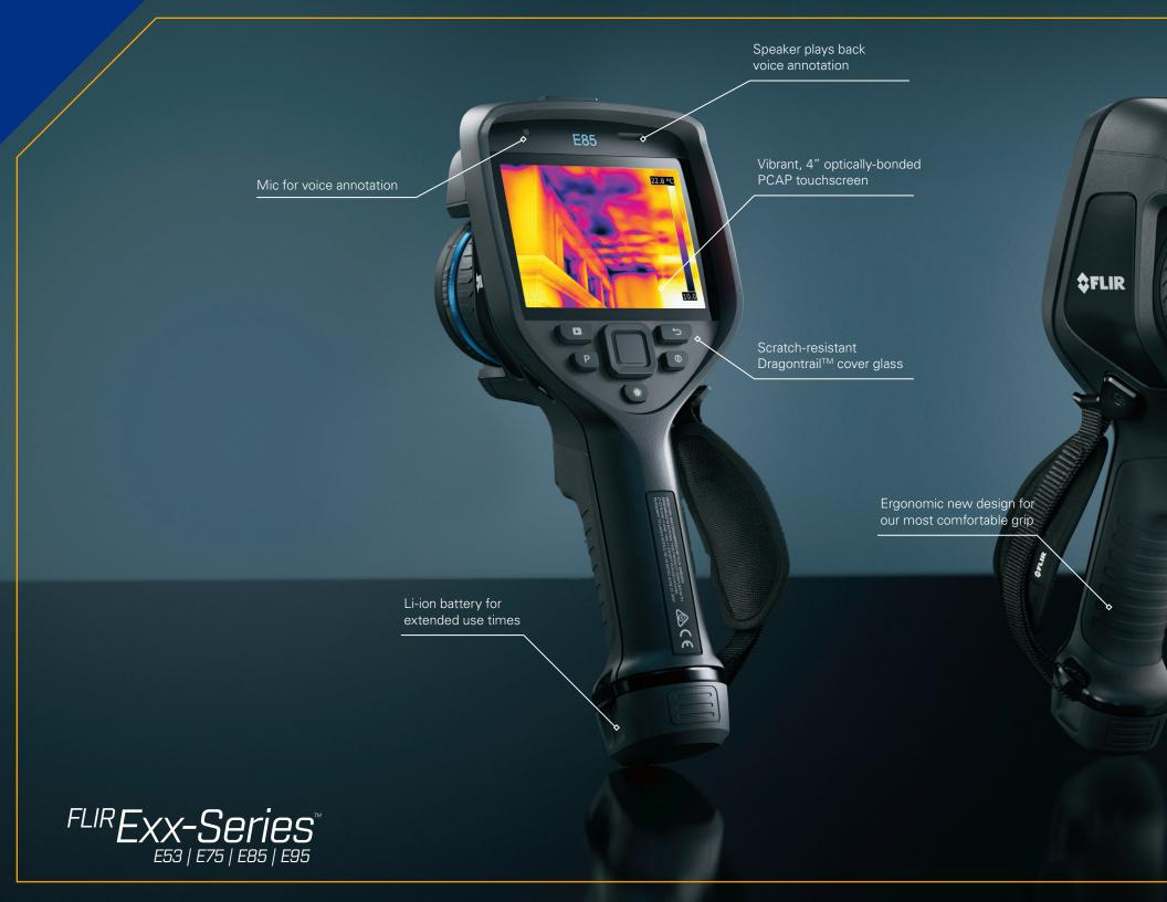
Laser provides distance measurement and precise autofocus\*
