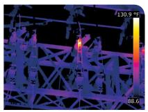
Overheating substation circuit breaker
