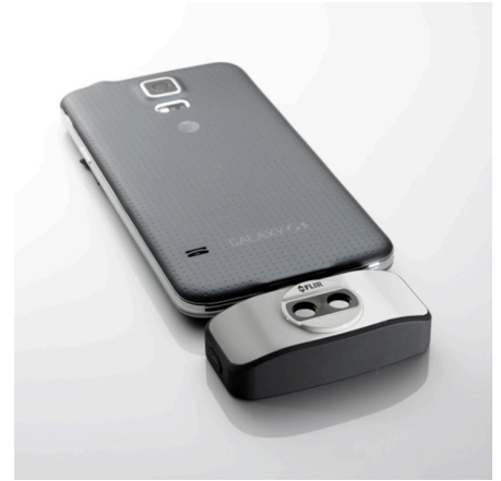
Figure 33.3 2015: FLIR One, an accessory to iPhone and Android mobile phones. Weight: 90 g (3.2 oz.).
