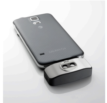
Figure 13.3 2015: FLIR One, an accessory to iPhone and Android mobile phones. Weight: 90 g (3.2 oz.).
