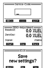
If zero point adjustment was not possible because the current gas reading is more than 25% of the measuring range due to a strong drift, the zero point can only be adjusted by qualified service personnel using the extended service code "0055" (factory setting) even with a deviation of up to 35% of the measuring range. It must be ensured that the sensor is in fresh air free of measuring gas or that zero gas is supplied to the sensor.
