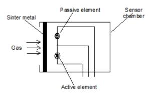
The passive sensor element is exposed to the same environmental conditions as the active sensor element and is used to compensate for environmental influences (e.g. temperature changes).
