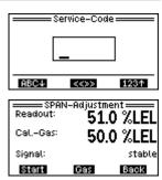
After pressing the middle button [Gas], the test gas concentration can be changed with the left or right button and stored with the middle button.
