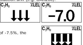
If the measuring signal falls below the measuring range of -7.5%, the arrows  $\downarrow\downarrow\downarrow$  appear permanently in the display.
