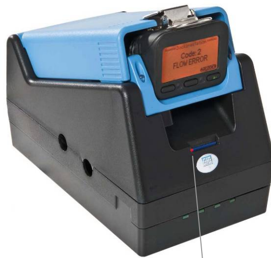
Bump test failed: Display is red + red LED lit in slot Display of the error which has occurred (shown here Code 2: Flow error)
