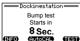
Bump test automatically starts after 10 seconds
