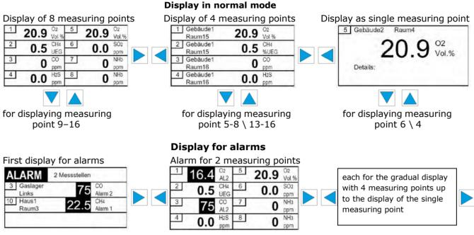
The display is backlit; the light intensity can be increased using any control button. In the event of a gas alarm or faults, the display lighting is automatically activated with a red background.
