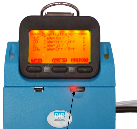
Bump test not successful: Display is red + red LED lit in slot Display of the error which has occurred
