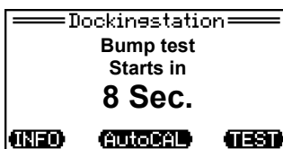
Bump test starts after 10 seconds automatically
