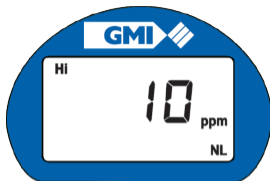
Fig. 2-4 Hi Alarm Level
