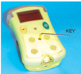
Fig. 4.1 Key in Cover Screw
