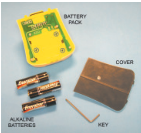
Fig. 4.13 Alkaline Batteries Removed
