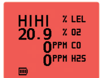
Red display in alarm conditions
