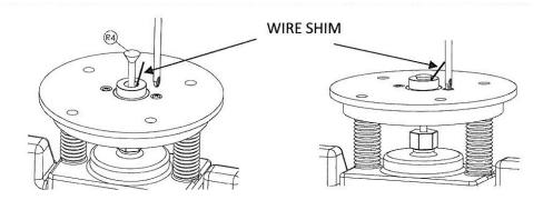
A practice cut with different size shims may be made to establish the preferred tightness or looseness of the fit. Of course, as an alternative, the tenon may be sanded down to establish the desired fit as well.
